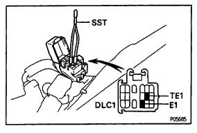
Using SST, connect terminals TE1 and E1 of the data link connector 1.
