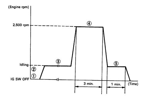
HINT: When start this test, coolant temp. is 35°C (95°F) or less and A/C switch OFF. Before this test, check the feedback voltage for oxygen sensor.
