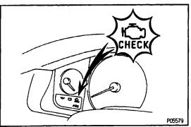
Read the diagnostic trouble code as indicated by the number of flashes of the "CHECK" engine warning light.
